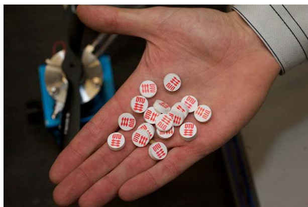
Fig. 2. Tablets of hexaamminemagnesium chloride (featuring the logo of the Technical University of Denmark) can be handled conveniently in the palm of a hand. Each pellet is approximately 1\text{ cm}^3 in size, contains \sim 0.62\text{ g NH}_3 and correspondingly 0.11\text{ g} of pure hydrogen. The hydrogen content is roughly 1.3\text{ l} gaseous \text{H}_2 (STP). This corresponds to a virtual hydrogen pressure of about 1300\text{ bar} in the tablets.
