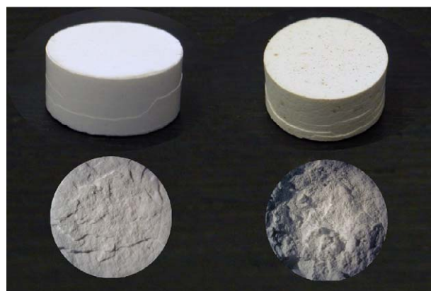
Fig. 3. Upper left: original tablet of \text{Mg}(\text{NH}_3)_6\text{Cl}_2 prior to ammonia desorption. Lower left: tablet broken into half before ammonia desorption. Upper right: original tablet of \text{Mg}(\text{NH}_3)_6\text{Cl}_2 after ammonia desorption. Lower right: tablet broken into half after ammonia desorption. The slight coloring of the tablet after desorption is due to impurities introduced from the sample holder.
